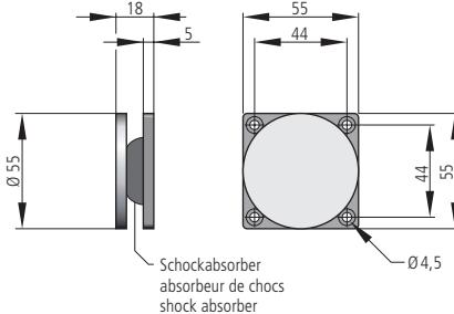
Flexibler Anker/Induit flexible/flexible doorplate AFS 55
