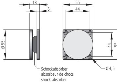
**Flexibler Anker/Induit flexible/flexible doorplate AFS 55**
