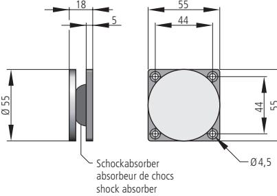
**Flexibler Anker/Induit flexible/flexible doorplate AFS 55**
