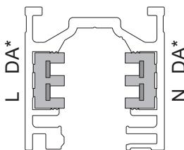
**EN** The adapter or track box of this luminaire/spotlight may **only be used in combination with the ZUMTOBEL L3 and DALI track and in DALI installations** corresponding with the diagram shown. Using these devices in tracks with standard 3-phase installations may damage the luminaire and is prohibited.
