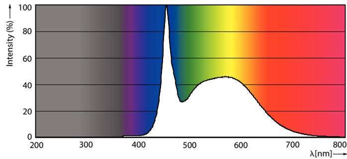
Spectral Power Distribution Colour - CorePro LED PLL HF 24W 865 4P 2G11
