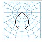
Belviso C1 625 CDP LED3900nw FB TX037990 C0 - C180 UGR I = 17,3 UGR q = 17,2 DIN 5040: A50 UTE: 1,00 C CEN Flux Code: 65 89 97 100 100
