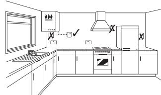
**GB** For best performance, install in an open space. Leave at least 30cm distance from any metal objects including wall boxes and boiler housing. **Do not mount on metal wall boxes.**
