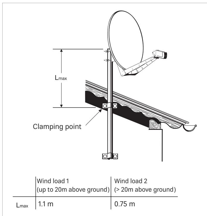
**If you arrange the structure differently you must calculate wind loading and bending moment at the clamping point as specified in DIN EN 60728-11 (or have a specialist do the calculation for you).**
