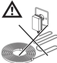
Do not connect the rope light to the supply while it is wound onto a reel.
