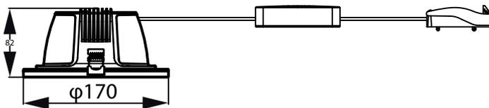
Cut-out hole diameter - Ø150mm
