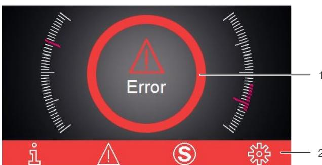
Fig. 36: Screen in the event of a malfunction
