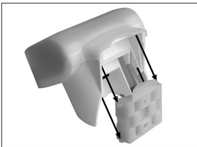
Push the housing into the installed bracket from above. The tabs on the bracket must engage in the rails of the housing.
