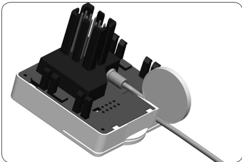
1. Carefully pull the operating unit off the installation housing.
