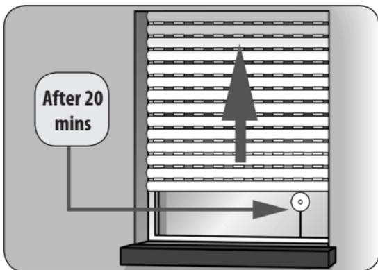
After approx. 20 minutes, the roller shutter is automatically raised a small amount to uncover the sensor. If the sun continues to shine, then the roller shutter remains in this position. If the brightness decreases below the set limit, it returns to the upper end point.
