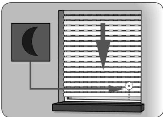
At dusk, the roller shutters will lower to the lower end point after approx. 15 seconds. The roller shutters will open again once the configured opening time is reached or in the event of a manual UP command.
