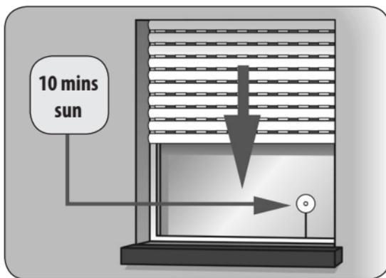
If the sensor detects uninterrupted sunlight for 10 minutes, the shutter will descend until its shadow covers the light sensor.
