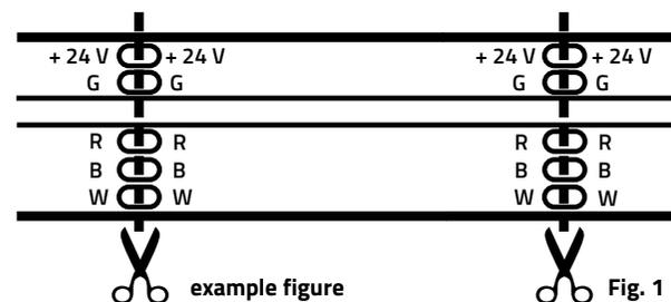
Separate the VARDIFLEX LED strip at the marked position. For a tightly assembled LED strip is a micro side cutter or an optional cutter required.
