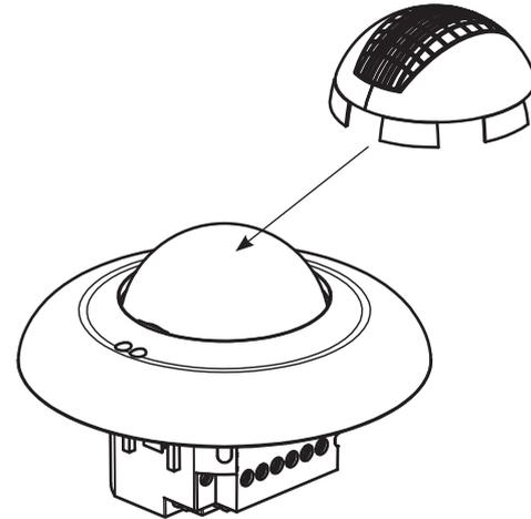
In case the sensing area is too large or areas are being covered that should not be monitored, the range can be reduced or limited through use of the enclosed masking clips.
