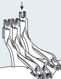
If several FFKu-Fibre net require rerouting, as many Fibre net IB as required can be stacked on top of each other. Push the following Fibre net IB from above into the locking mechanism of the Fibre net IB already installed, and interlock at the bottom. The interlocking mechanism on Fibre net IB is detachable.
