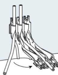
FFKu-Fibre net can be subsequently placed into the Fibre net IB already installed or removed again.
